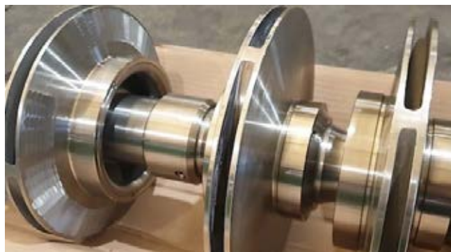
» Rotor centrifugalne crpke a AM rotorima u servisu Baker Hughes Bari u Italiji
