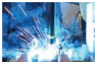
» Kontroliran prijelaz materijala - Controlled modified short arc
